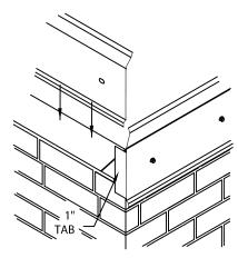
STEP 3 - RAIL MITER PREPARATION SEE PAGE 4 FOR MITER PREPARATION. FASTEN MITER BASE RAIL TO NAILER(S) THROUGH BASE RAIL SLOTS WITH PROVIDED FASTENERS.
